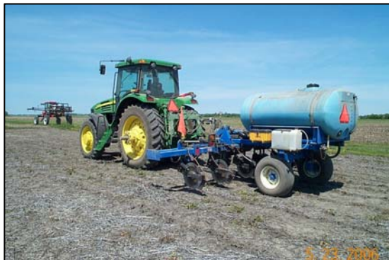
Applying pre-plant treatments with the JD 7920 and DMI 2800 UAN applicator
