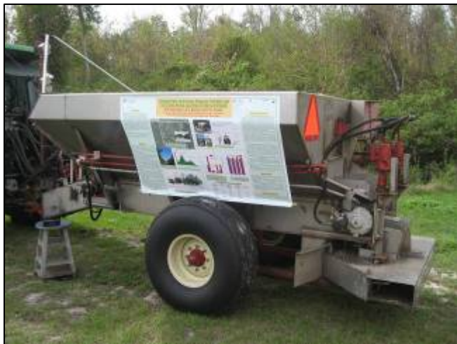
Sensors mounted on the mast between the tractor and fertilizer spreader provide tree size information to vary fertilizer rates (image courtesy Balaji Sethuramasamyraji).
