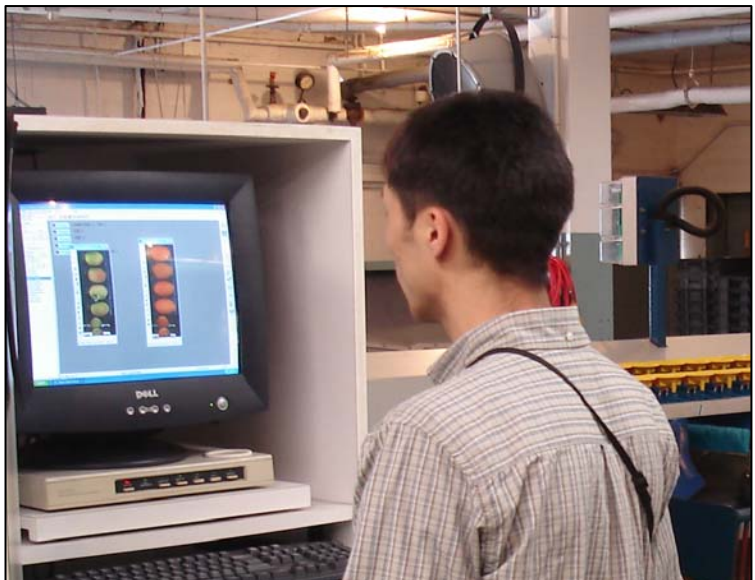
The Citrus Center staff demonstrated how fruit can be individually analyzed by spectral sensors to categorize for optimal marketing (image courtesy Harold Reetz).
