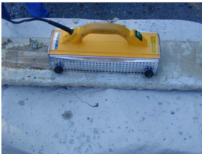
Silent Paint Remover in contact with a difficult to chemically strip painted board
