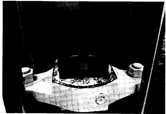
Figure 2. — Photograph showing the apparatus used to hold the edge withdrawal specimens during testing.
