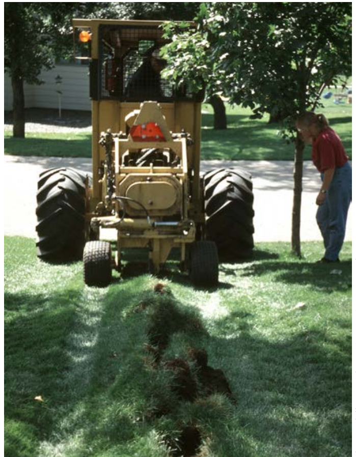
Figure 7. This trenching operation is designed to cut root grafts between trees.
